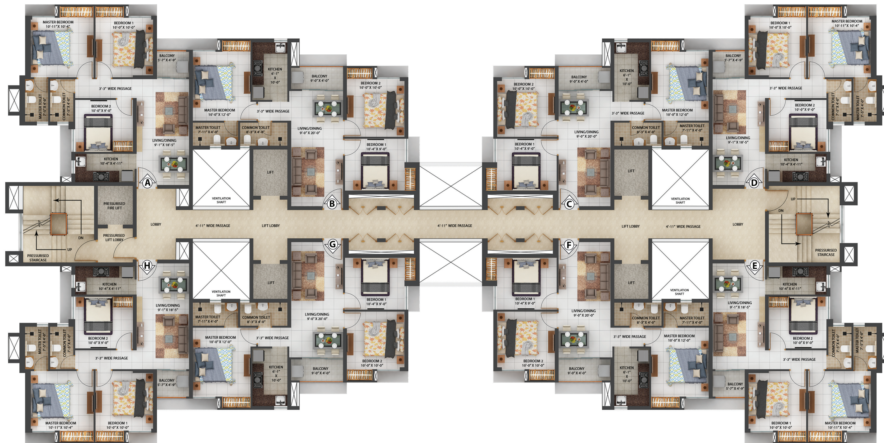
BLOCK B5, B6, B7 (2B+G+27) | Typical Floor Plan - 5th to 27th Floor
